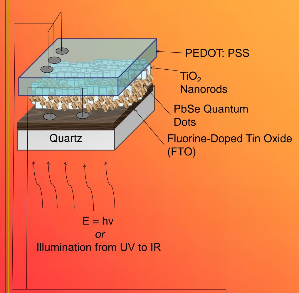
Collected light is used to calculate the external quantum efficiency; *I-V* characteristics are studied.
