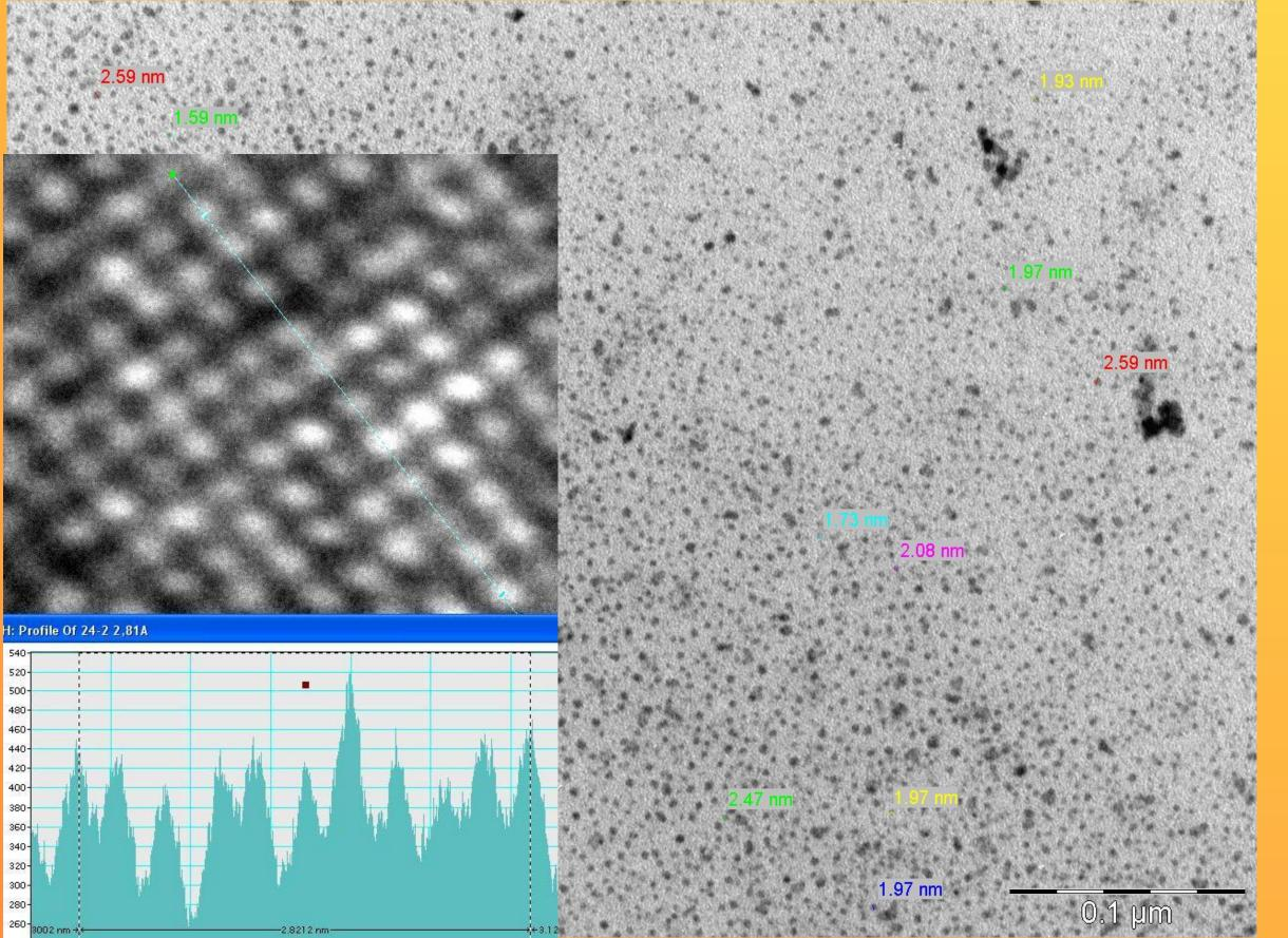
Scanning Electron Microscope Image of the PbSe quantum dots grown to an average diameter of 2 nm, which corresponds to a conduction band off-set of 0.35 eV, a value which will facilitate the electron injection into and ballistic transport through the  $TiO_2$
