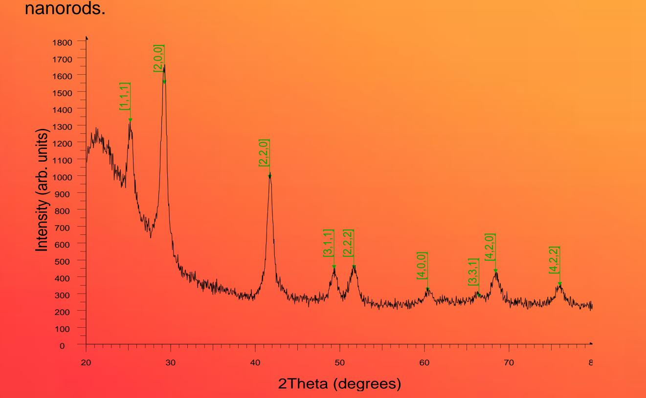
X-Ray Diffraction Pattern for the PbSe quantum dots showing the crystalline result of the novel growth process.
