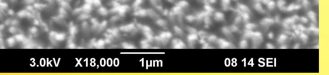
Titanium Dioxide nanorod  $(TiO_2)$  image taken with a scanning electron microscope. The  $TiO_2$  nanorods are a good choice for the construction of solar cells due to the very large surface area they present relative to typical *pn* junction cells. Inset elucidates the average  $TiO_2$  nanorod length of 2 µm, with 180 nm diameters. The density of the nanorods is controlled in order to yield the maximum monolayer coverage with the PbSe quantum dots.
